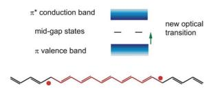
Fig. 3. Schematic illustration of a region of reversed sense of bond alternation on a *trans* polyacetylene chain, with soliton-like topological defects to either side. The associated electronic structure (for p-doped material) is shown in the band scheme.
