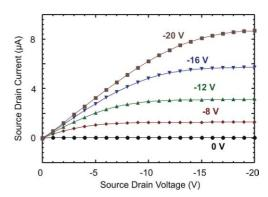
Fig. 2. Electrical transfer characteristics for polyacetylene transistors as shown in Fig. 1. The source-drain separation (channel length) is 5  $\mu$ m, the channel length is 90 cm (interdigitated electrodes), and the SiO<sub>2</sub> thickness 200 nm.
