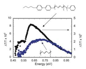
Fig. 4. Extra optical absorption due to field-induced charge in a polyacetylene field-effect structure versus photon energy. Data are shown for both the standard form of Durham polyacetylene and for polyacetylene with biphenyl chain ends.
