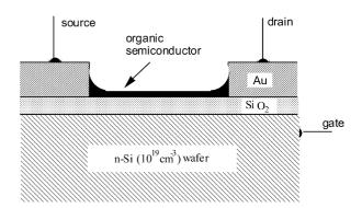
Fig. 1. Structure of a Field-Effect Transistor, fabricated using a top layer of Durham polyacetylene on a  $SiO_2$  dielectric layer, with gold source and drain contacts. The doped Si wafer acts as substrate and gate.
